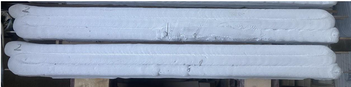
Fig. 8. Beams made by 3D printing with reinforcement with single bars after reaching the design strength
