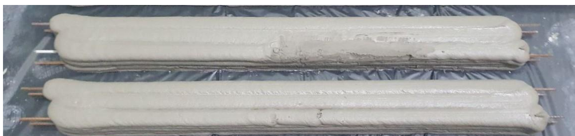
Fig. 6. Reinforced concrete beams printed by 3D printing with reinforcement by single bars
